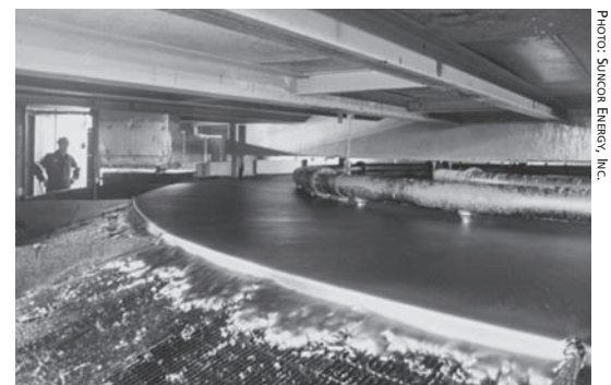
A separation cell is one step in the extraction of bitumen from tar sands mixed with water.
